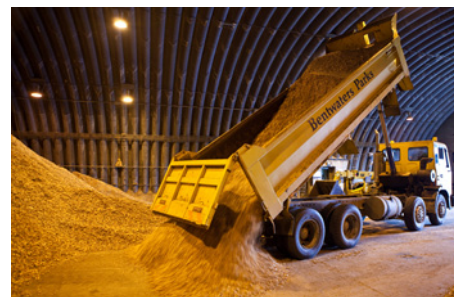
Freshly produced woodchip being delivered to a store for further drying at Eastern Woodfuel.
