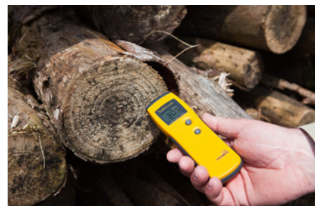
Testing the moisture content of seasoned wood.
