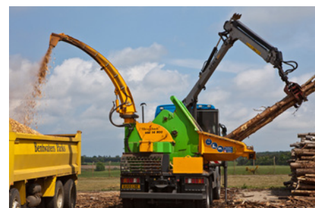
Seasoned logs being chipped by Anglia Woodfuels to produce wood-fuel
